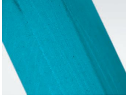
O-Ring following traditional deflashing methods with probable leak paths
