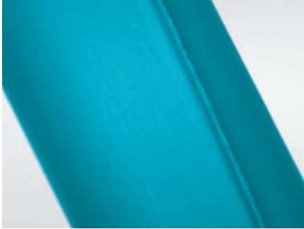
O-Ring without surface and deflashing treatment showing flash
