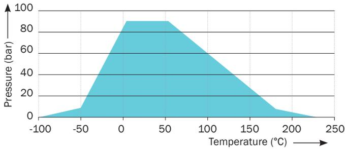
The temperature and pressure recommendations in the graphs apply to gaskets with a thickness of 2.0 mm and smooth flanges. Higher stresses are possible when thinner gaskets are used.
